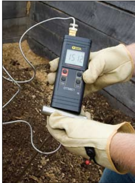
Figure 1. One example of a moisture probe. (Notice the temperature of 151°F.)
